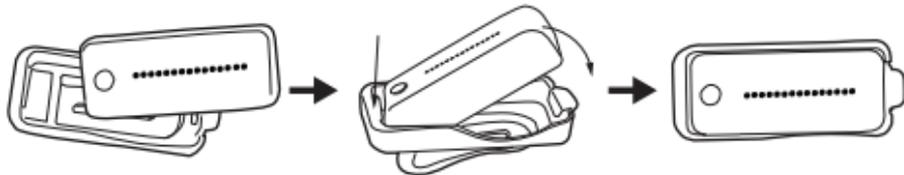
Place one end of the [MU] into the Clip and snap the other side into place.
